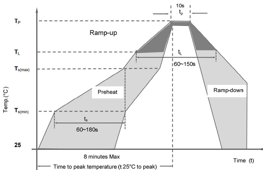
Figure 9. Reflow Soldering
