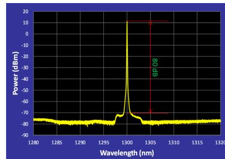
TLS-1000 tunable lasers are new-generation high performance continuous wave (CW) tunable laser sources for use in various single band or combined band windows, ranging from 1050 nm to 1660 nm. The innovative design employs the state-of-the-art tunable technology and gain continuation in wide wavelength range. With no moving parts, the voltage-controlled wavelength tuning enables rapid wavelength switching over the whole operating wavelength window.
